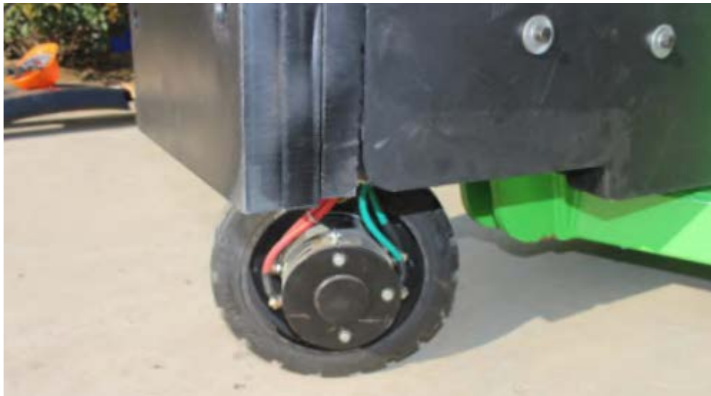
Electric Driving Wheel: rear axle drive and electromagnetic brake(250x80mm)
